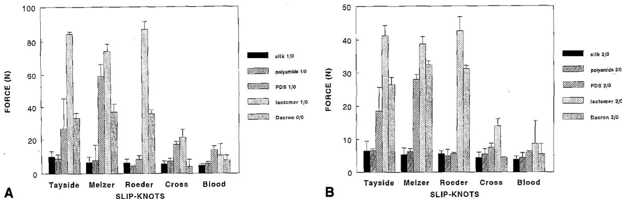
**Fig. 8.** a Bar graph of the median forces (and third-quartile range) in Newtons required to initiate reverse slippage of the slipknots formed in size 1/0 or 0/0 of the suture materials. b Bar graph of the median forces (and third-quartile range) in Newtons required to initiate reverse slippage of the slipknots formed in size 2/0 of the suture materials.
