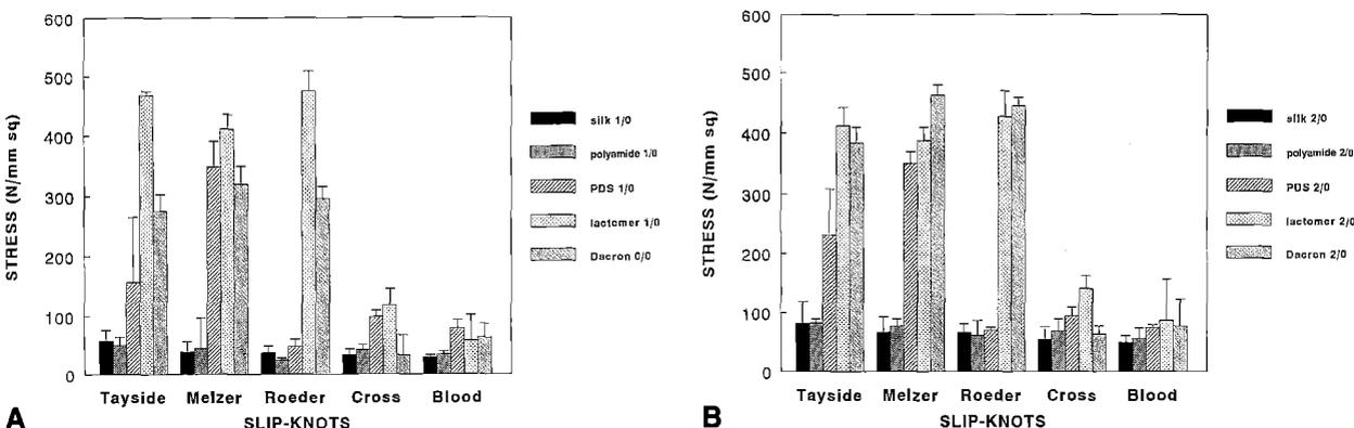
**Fig. 9.** a Bar graph of the median stress (and third-quartile range) in Newtons/mm<sup>2</sup> required to initiate reverse slippage of the slipknots formed in size 1/0 or 0/0 of the suture materials. b Bar graph of the median stress (and third-quartile range) in Newtons/mm<sup>2</sup> required to initiate reverse slippage of the slipknots formed in size 2/0 of the suture materials.
